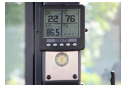
New information display in the B-column for the exhaust gas system for 8600 and 9600 series loaders
